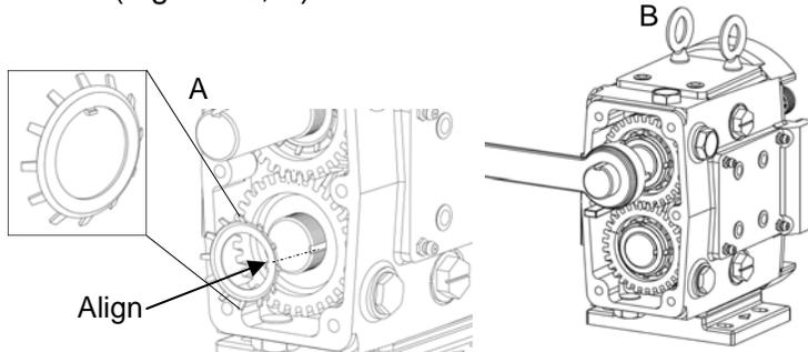
**Figure 58: Installing Lock Washer and Lock Nut**
