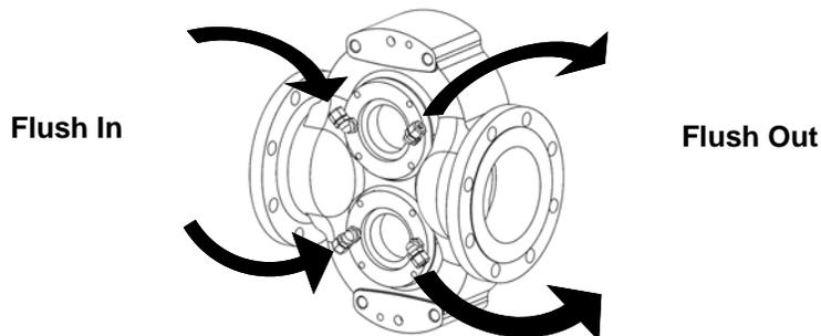
Figure 15: Proper Flushing for XP Double Seal
