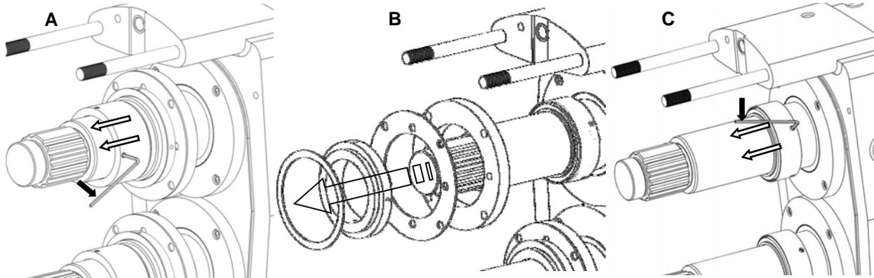
Figure 40: XP Double Mechanical Seal Disassembly
