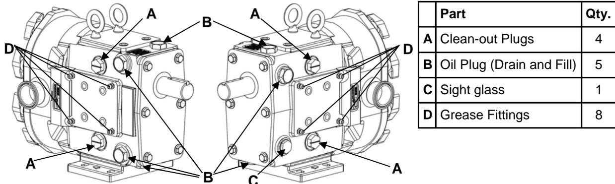
Figure 16: Lubrication Points
