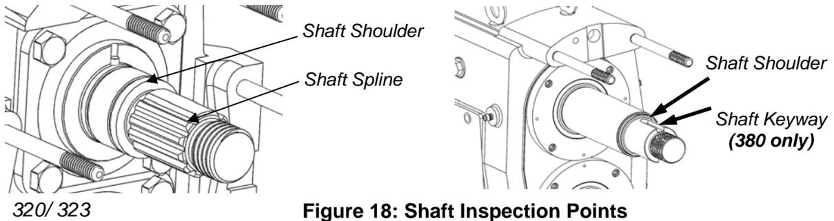
**Figure 18: Shaft Inspection Points**
