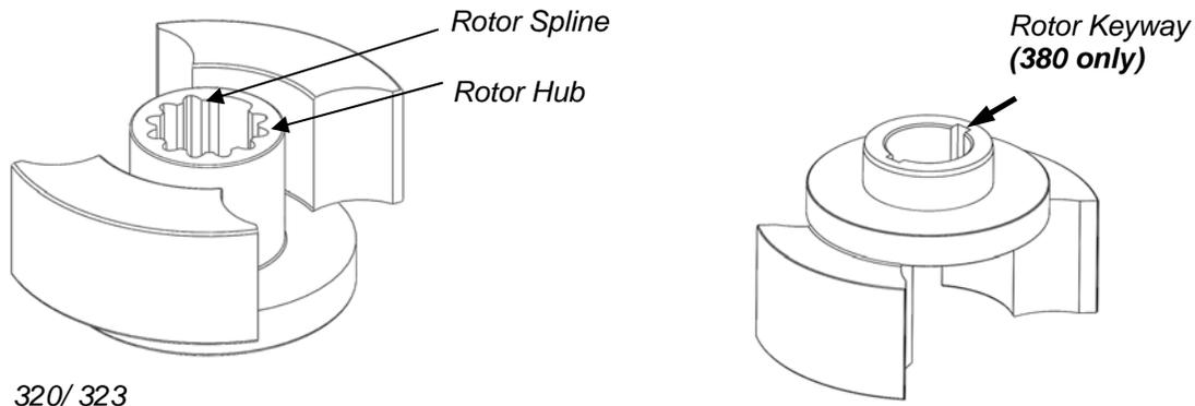
**Figure 19: Rotor Inspection Points**
