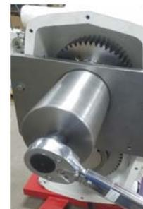
5. Remove the timing gears and the timing gear keys. The gears should slide off the shafts. If a gear puller is required, three tapped holes are provided in each gear for that purpose.
