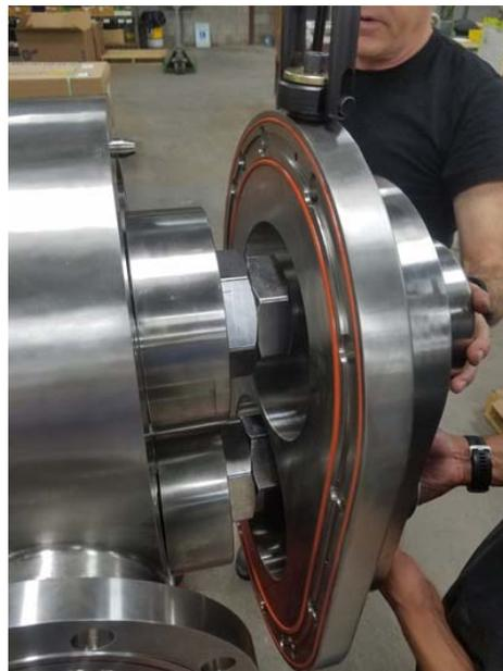
**ROTOR REMOVAL PROCESS - FLUID END DISASSEMBLY**
