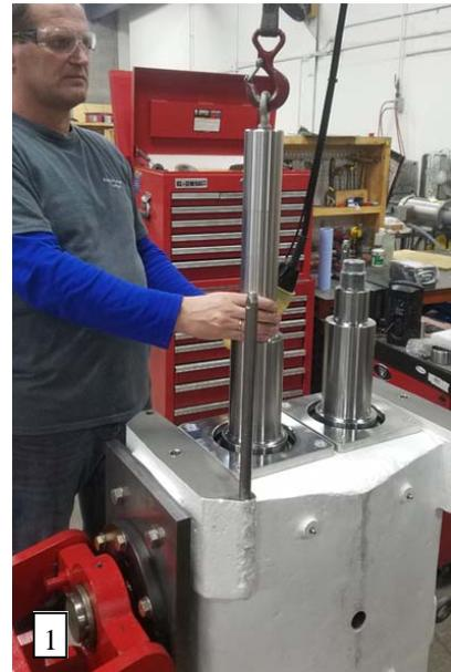
5. **NOTE** - Before moving forward, critical measurements must be made to determine the need for a bearing shims.
