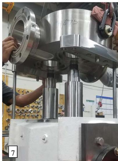
**MECHANICAL SEAL REMOVAL - FLUID HEAD DISASSEMBLY**
