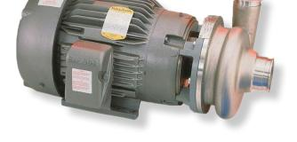
The DV Series, with a unique double volute design, is ideally suited for CIP return applications. The double volute design reduces air binding without an air relief valve at half the cost of a self-priming pump.
