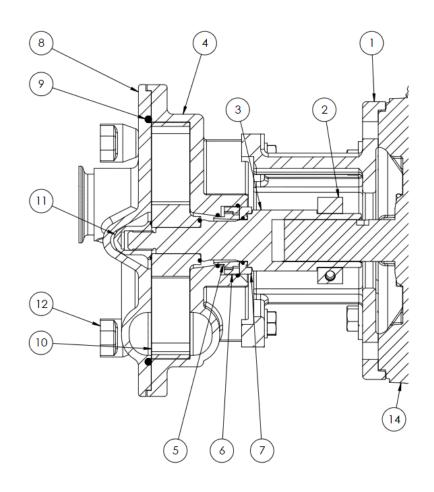
SP Series Pump Component Breakdown
